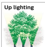
An unnatural, therefore dramatic way of lighting trees and architectural structures. Highlights details on structures and can be used to repeat patterns to create interest.
