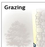
Enhances texture of a surface by positioning a fixture close to the surface and aiming the beam upward or downward.
