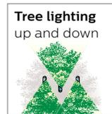
**Tree lighting up and down** Combines simulated full moon light filtering through the tree and uplighting from within to illuminate the canopy. Creates a softer light on the trunk and keeps all fixtures off the ground.
