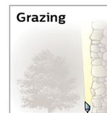
**Grazing** Enhances texture of a surface by positioning a fixture close to the surface and aiming the beam upward or downward.
