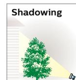
**Shadowing** Creates a shadow on a vertical surface by placing the fixture in front of the subject.
