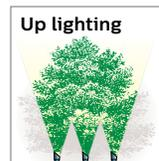
**Up lighting** An unnatural, therefore dramatic way of lighting trees and architectural structures. Highlights details on structures and can be used to repeat patterns to create interest.
